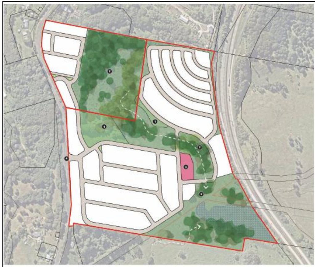
Figure 9: Site layout plan from the RPS urban design report shows an open space and drainage corridor running north – south through the site
