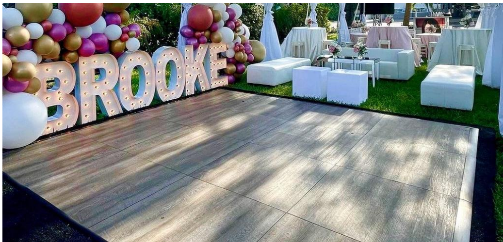
Figure 4: Typical removable dance floor (made from individual polypropylene panels, with timber-look finish that are light weight and clip together) - Photo from www.snaplockdancefloors.com .
