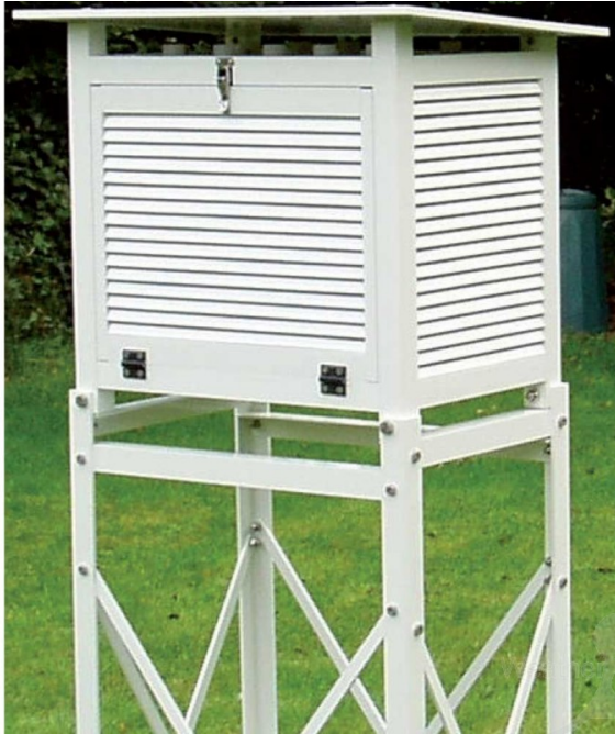
Figure 3: A Stevenson Screen in which instrumentation is housed
